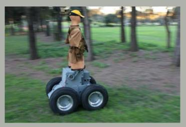
Marathon smart targets are intelligent armoured robots which can move freely across the entire training environment.
