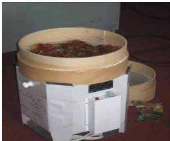
Saffron electric dryer introduced recently in Herat Province, Afghanistan
