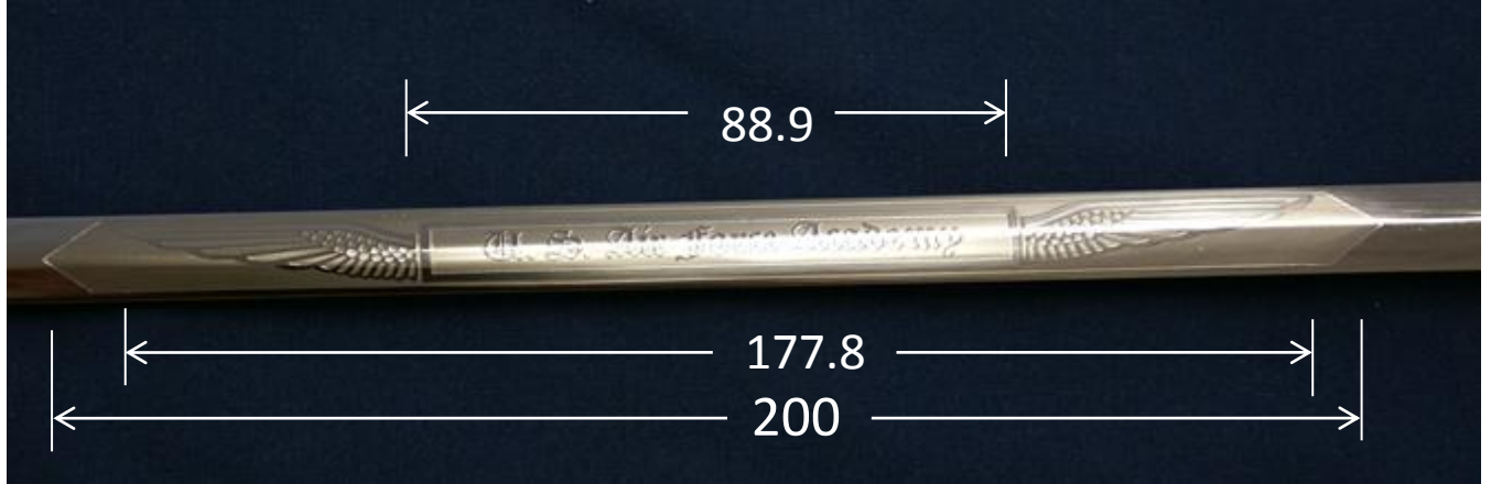
FIGURE 1 Blade Etching Design and Dimensions
