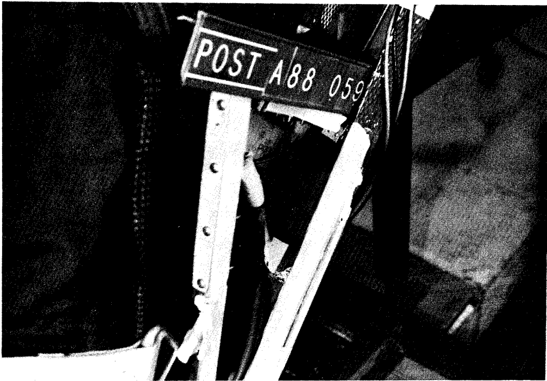
Figure 25. Failure of BL 20.3 right outboard brace tube anchorage to floor.
