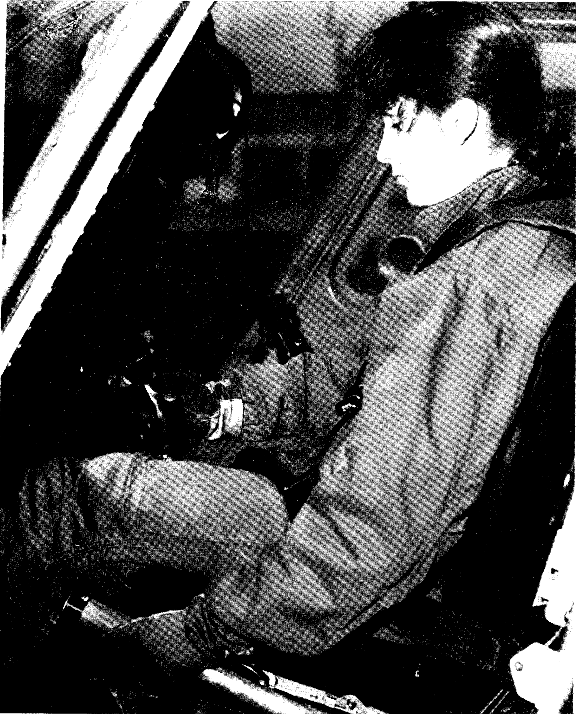
Figure 32. View of small female pilot in serial 71-20778 with five-point harness and seat pan BRP at 0.97 inch below sled test value (note collective in lowest position).
